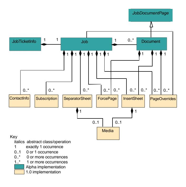
Figure 1.0 JTAPI High Level Model – Part 1
